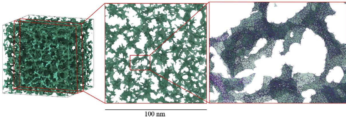
*Silica aerogel obtained by molecular dynamics simulation [1]. Right, zoom on the ligaments, brick of the silica aerogels structure*
