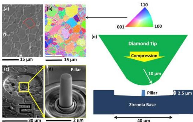
*Fabrication of a micro-pillar within one grain with a pre-selected orientation (Figure taken from Zeng et al. Acta Materialia, Volume 116, 2016, Pages 124-135)*
