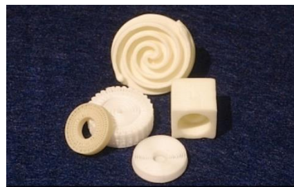
Parts produced by 3D extrusion of (a) ceramics and (b) tungsten carbide.
