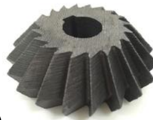
Parts produced by 3D extrusion of (a) ceramics and (b) tungsten carbide.
