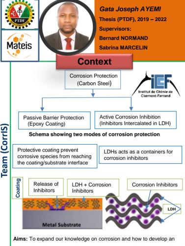
improved coating system for corrosion protection of carbon steel through
