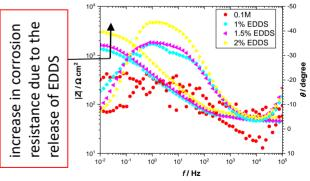
EIS Diagrams for bare carbon steel electrode for three LHD-EDDS concentration after 2h of immersion in 0.1M NaCl
