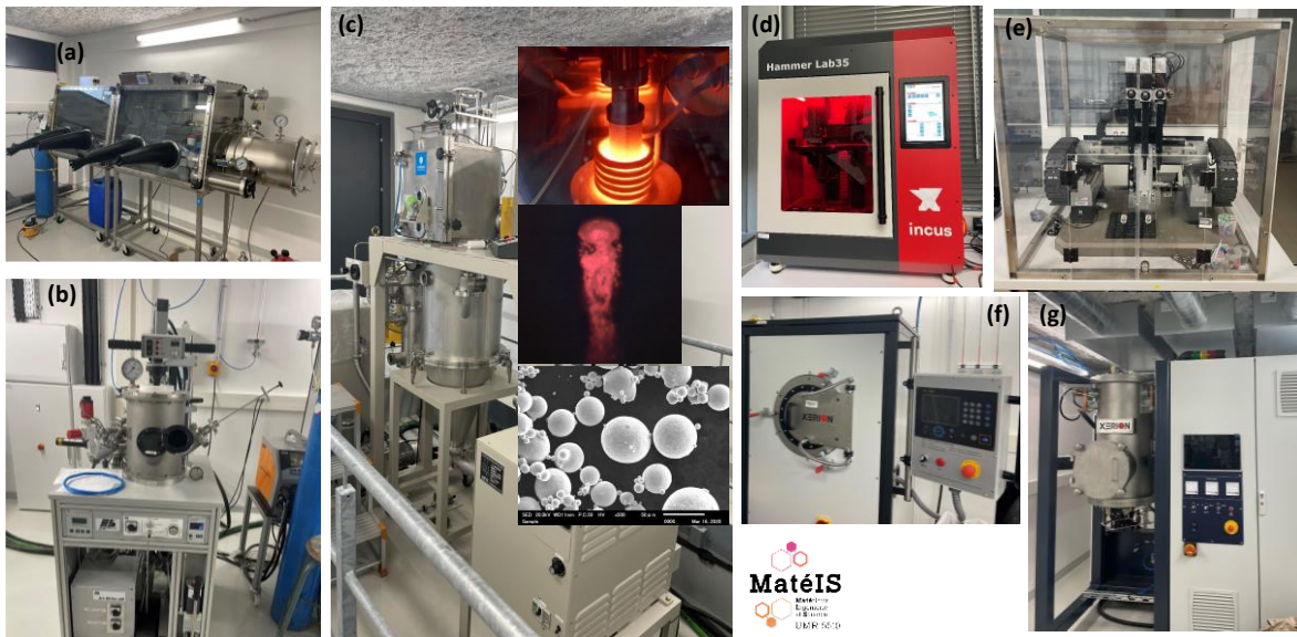
Glove box (a), Arc melter (b), Atomisation unit (c), Lithography(d), Robocasting (e), Debinding furnace (f), Sintering furnace (g)
