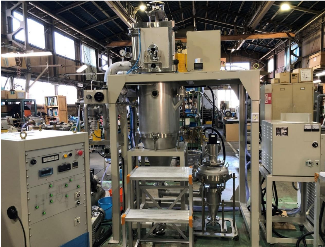
Small Atomisation Unit (200g / batch), Installed at INSA de Lyon / MATEIS
